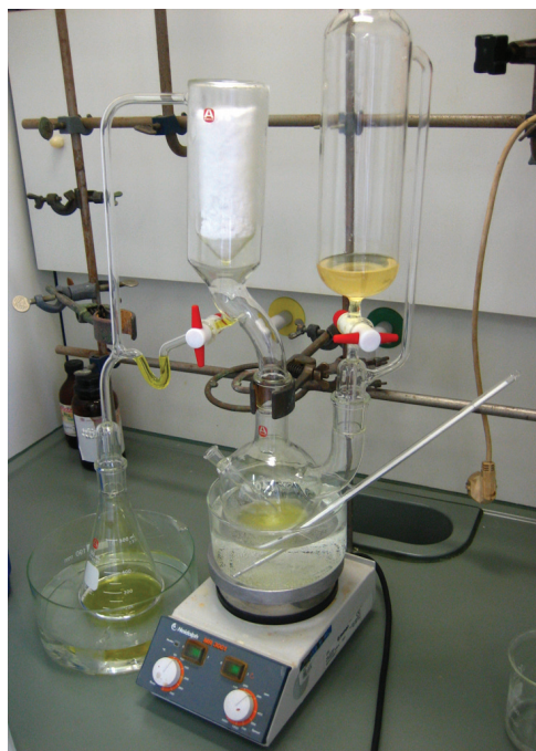
This apparatus for diazomethane preparation uses smooth-surface (not ground glass) joints to minimize the risk of explosion.
