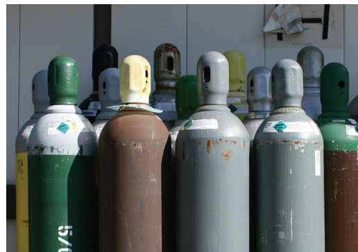
Securely cap gas cylinders when they are no longer in use.
