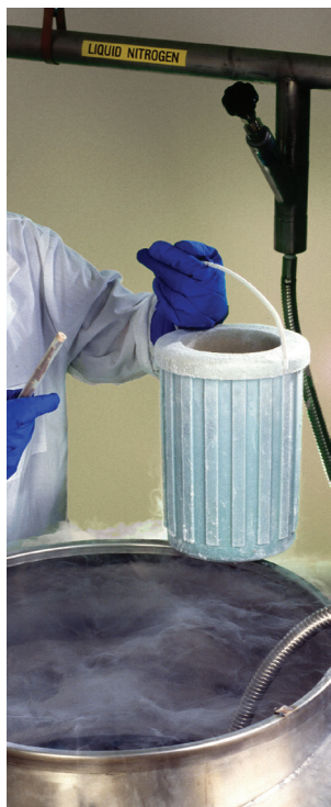
PPE for handling cryogens includes loose fitting thermal insulated or leather gloves, which can be easily removed.
