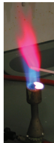
Any ignition source, such as this flame test for lithium salt, represents a potential source of fire.
