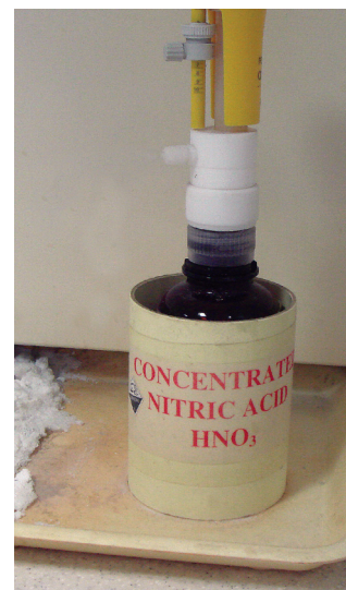
Corrosives such as nitric acid require protective wear, including corrosion-resistant gloves. Nitric acid is also an oxidant.
